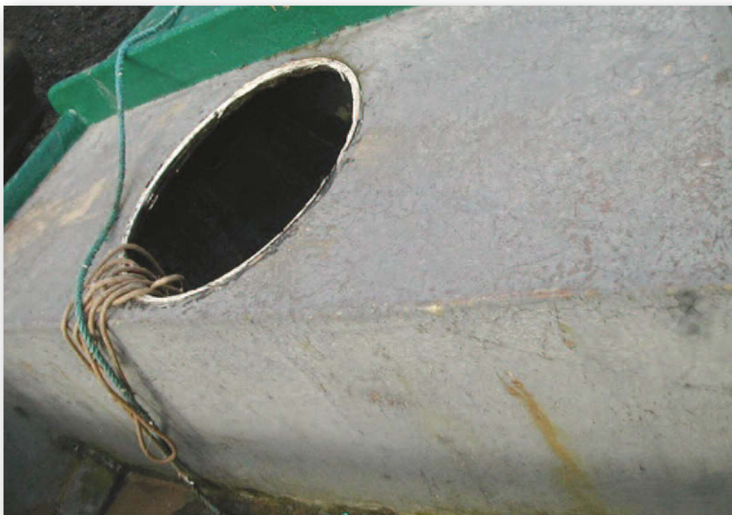
The for'd buoyancy chamber showing the missing inspection hatch and lid.
